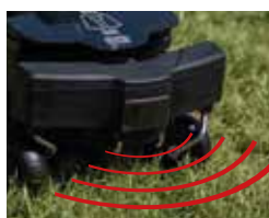
RADAR rilevamento ostacoli RADAR for obstacle detection
