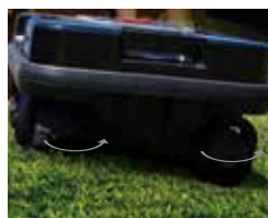
4 ruote motrici e sterzanti 4 driving and steering wheels
